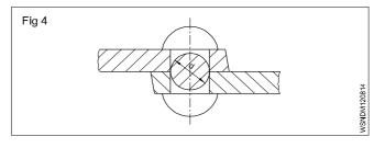
Rivet cross-section is the hole cross-section.
